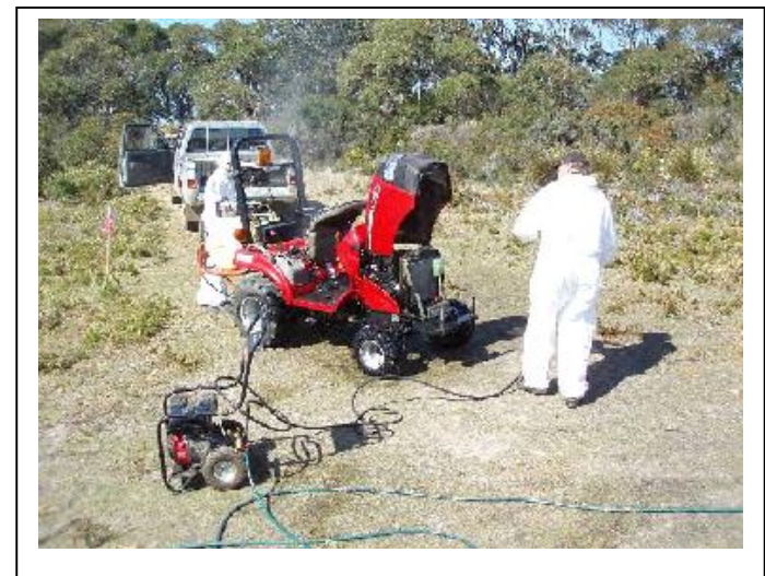
Portable high pressure water washdown of machinery
