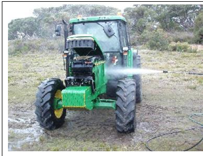
Portable high pressure water washdown of machinery
