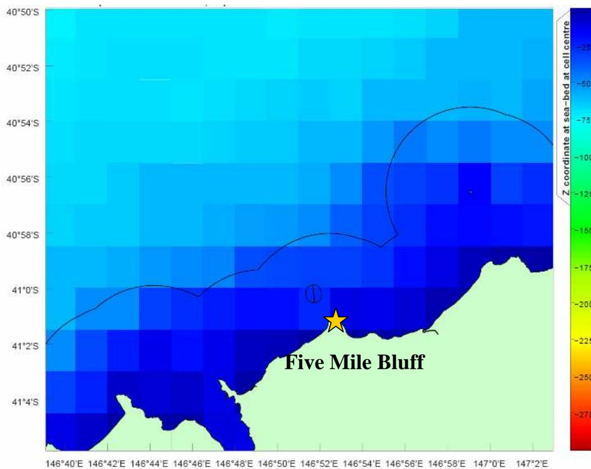
Figure 1 Location of the outfall pipe in the centre of the mixing zone (small ellipse), 2.7 km offshore Five Mile Bluff. Also shown is the boundary between State and Commonwealth waters.
