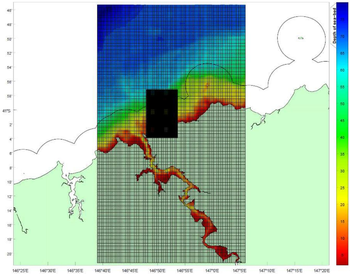
Figure 2(b) Proposed nested fine ( $0.0025^0$ ) and very fine ( $0.0005^0$ ) grid model domains. The boundary between Commonwealth and State waters is also shown.
