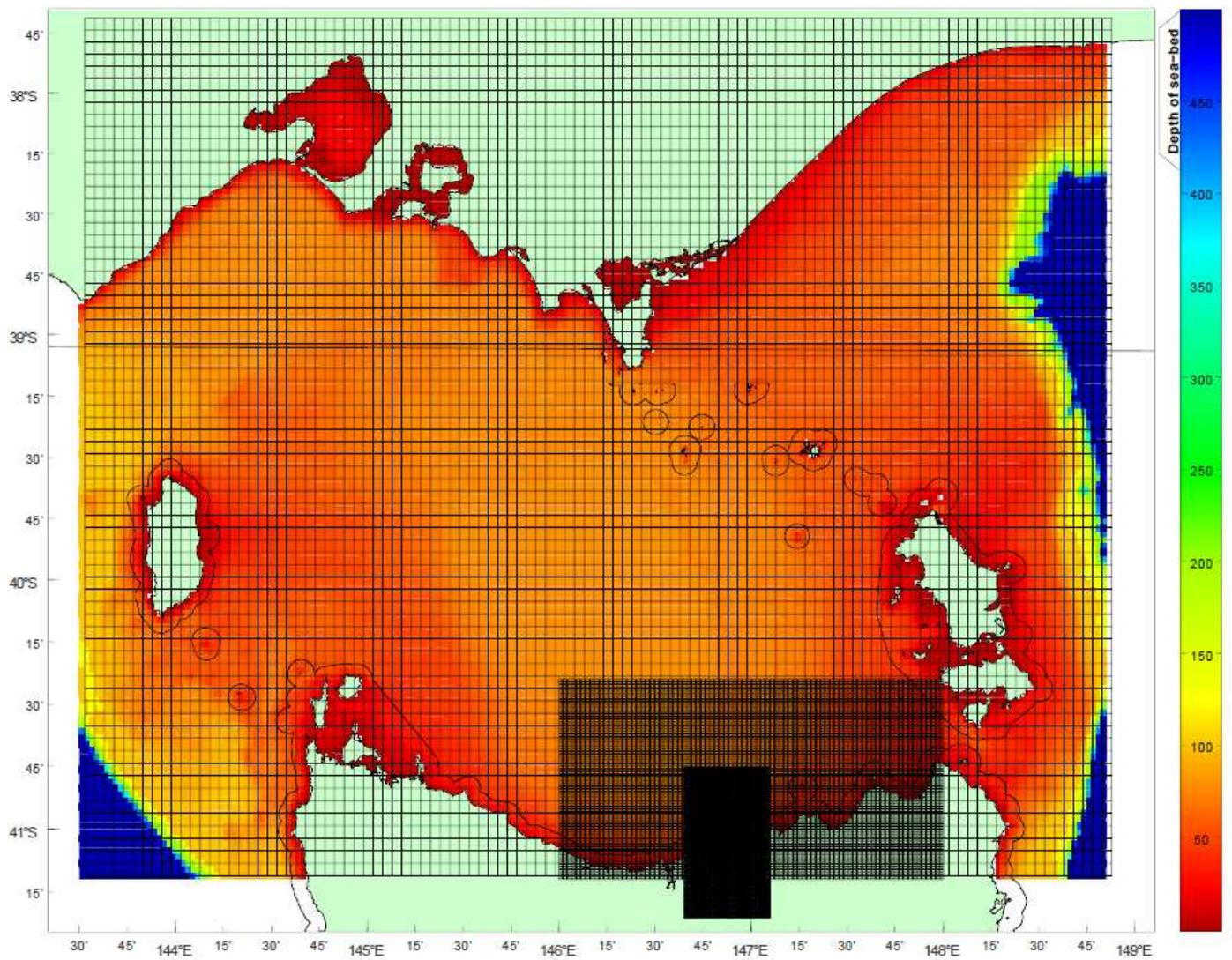
Figure 2(a) Proposed nested regional ( $0.025^{\circ}$ ), intermediate ( $0.01^{\circ}$ ) and fine ( $0.0025^{\circ}$ ) grid model domains. The boundary between Commonwealth and State waters is also shown.
