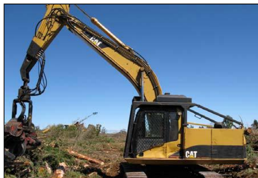
Excavator with cutting head
