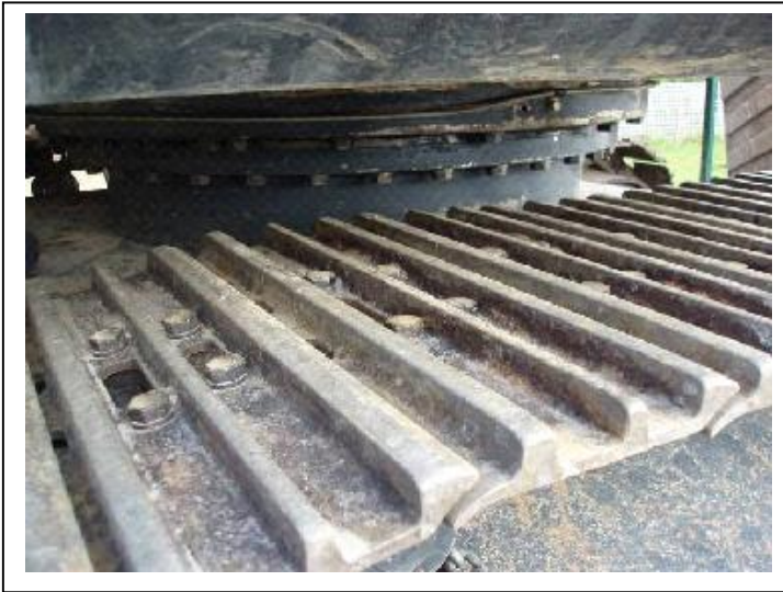
Steam cleaned excavator tracks prior to transportation to work site
