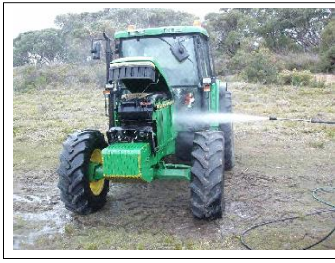
Portable high pressure water washdown of machinery
