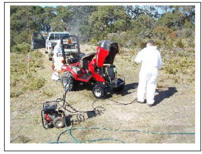
Portable high pressure water washdown of machinery
